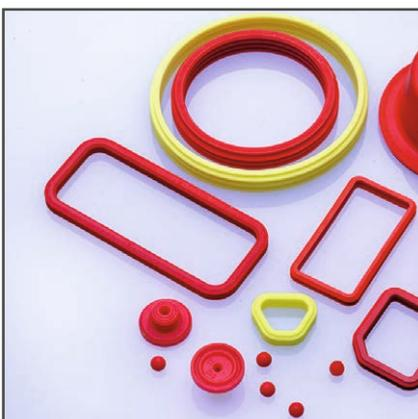
We designate **moulded parts** or **seals** as free-falling parts, which are **automatically manufactured** in middle to large quantities on **horizontal injection moulding machines**. After the tool opens, these parts are automatically demoulded from the cavity either by a brush and or push mechanism or by some other extraction system and then fall free into the provided transport container.
